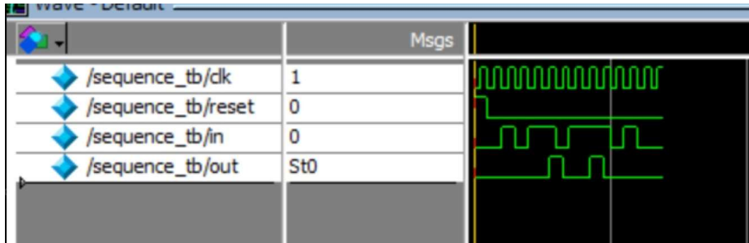
Figure 3.2: ModelSim Simulation Waveform — 1011 Sequence Detector
